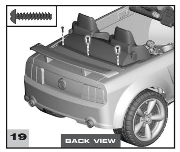
• Insert three black #8 x <sup>3</sup>/4" screws into the back of the seat and tighten.
